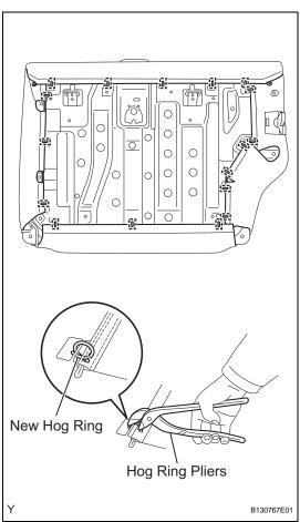
(b) Using hog ring pliers, install 17 new hog rings.
